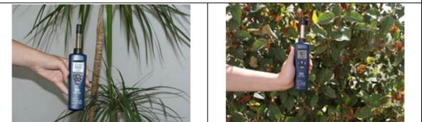
With the PCE-555 hydrometer you can measure ambient conditions including humidity in the top portion of the LCD and temperature shown on the bottom and also calculates wet bulb temperature and dew point, which are useful for calculating thermal stress.
