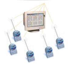
When pre-defined thresh-holds are crossed MicroLab sends an email or SMS alarm message automatically with the unit details.
